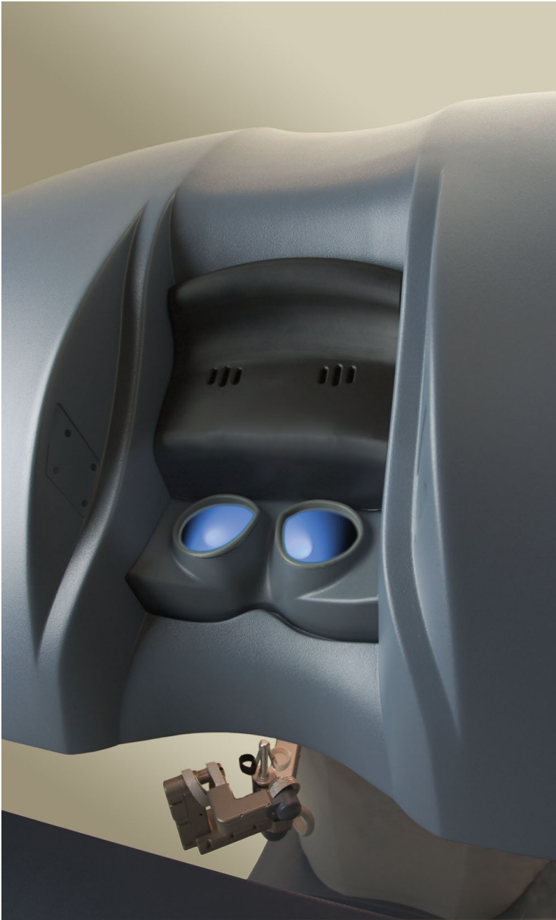
Surgeon console containing binocular stereoscopic screens
